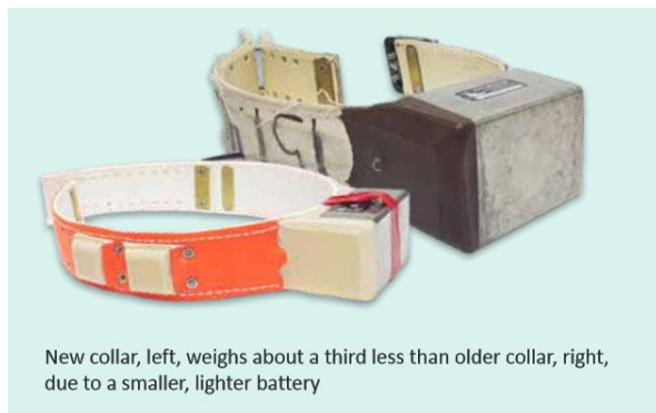
Figure 1: Many collars used today weigh 0.8 kg, much less than older collars, which weighed well over a kilogram. A snowmobile helmet, for comparison, weighs as much as 2 kg. (adapted from GNWT-ENR, n.d.)
